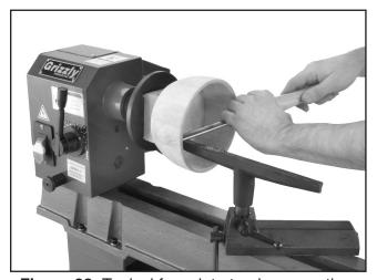
Figure 38. Typical faceplate turning operation.
